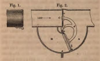
Fig. 1 is the *exit* separating valve, or that, at the end of the section nearest to its steam engine; this valve is opened by the compression of air caused by the piston after it has passed the branch which communicates with the air-pump.
